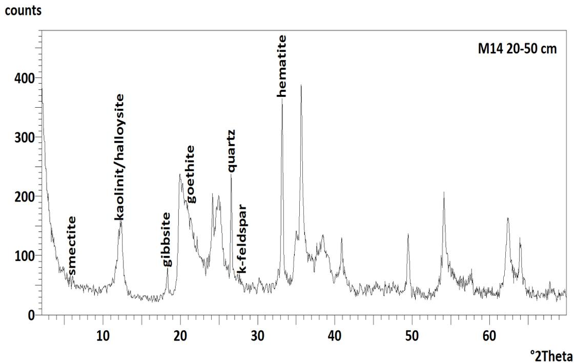
Figure 25. XRD diffractogram for sample M14 shows 1:1 kaolinite dominance
