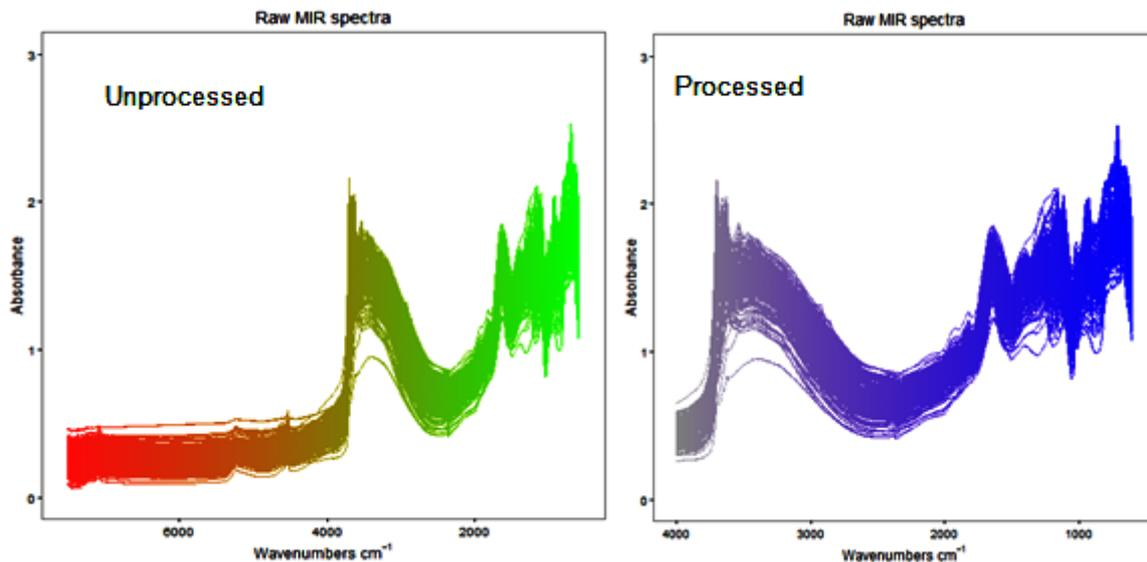
Figure 14. Unprocessed and processed MIR absorbance spectra to 4000-400 cm<sup>-1</sup>
