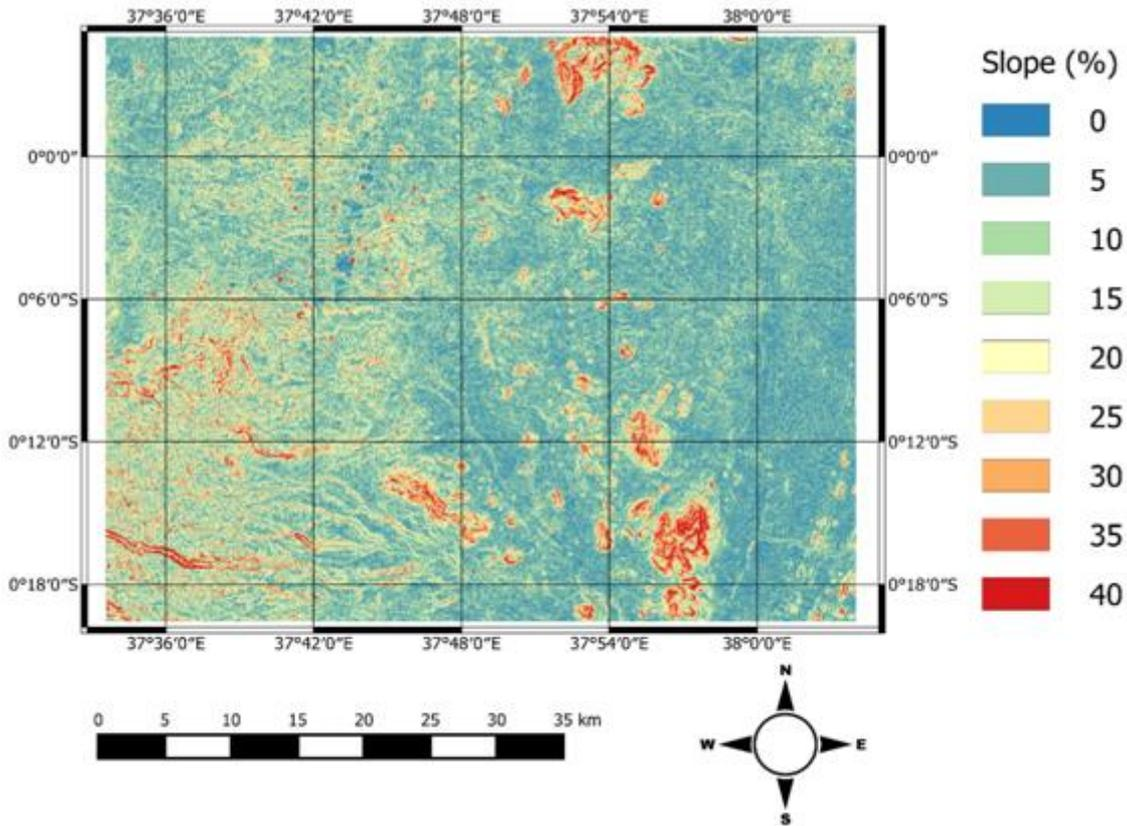
Figure 10. Slope percentage layer generated from DEM
