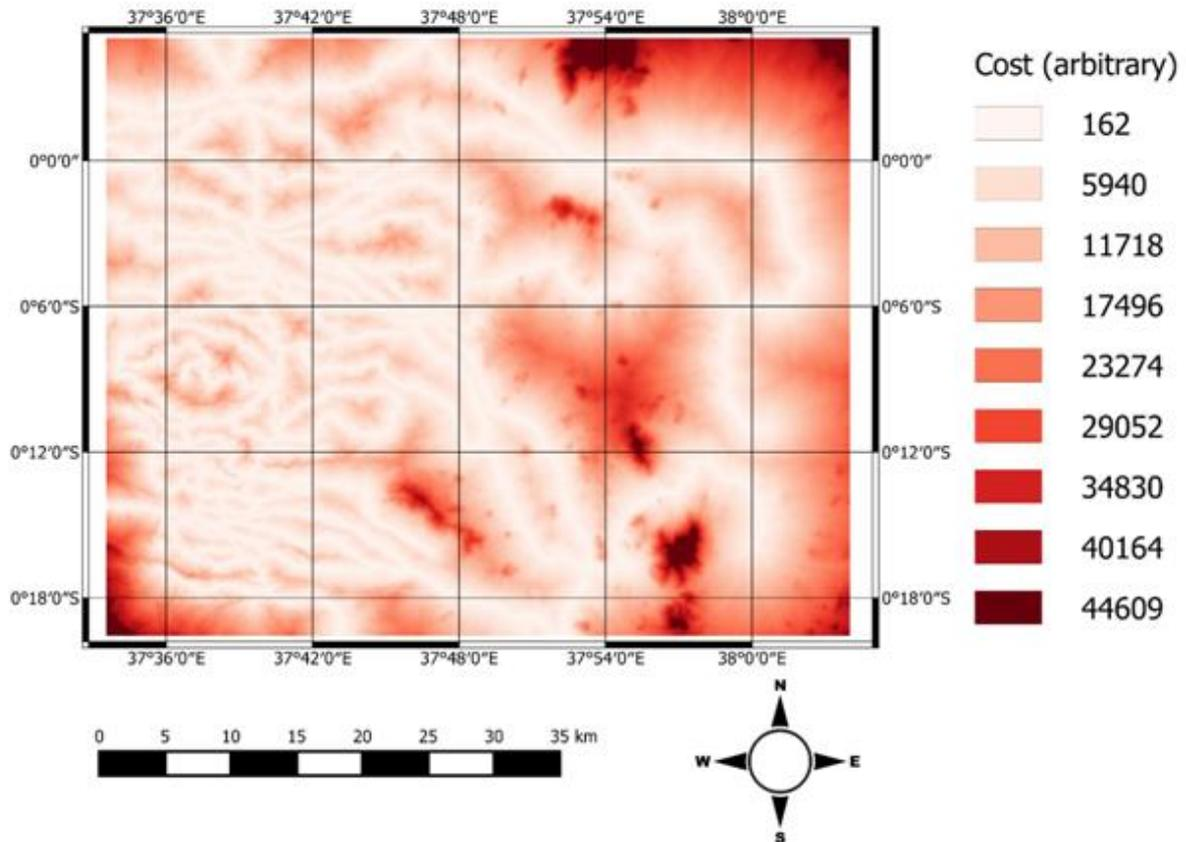
Figure 11. The cost of reach layer showing arbitrary cost units.
